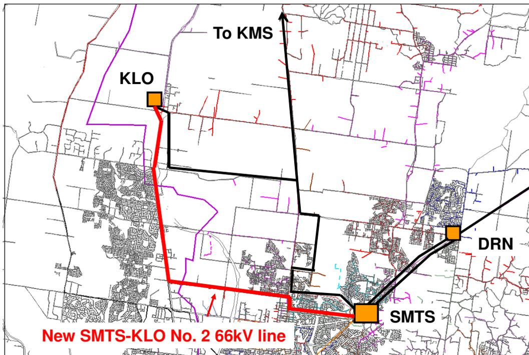
Figure 2 – SMTS-KLO/KMS No. 2 66kV line alternative route.
