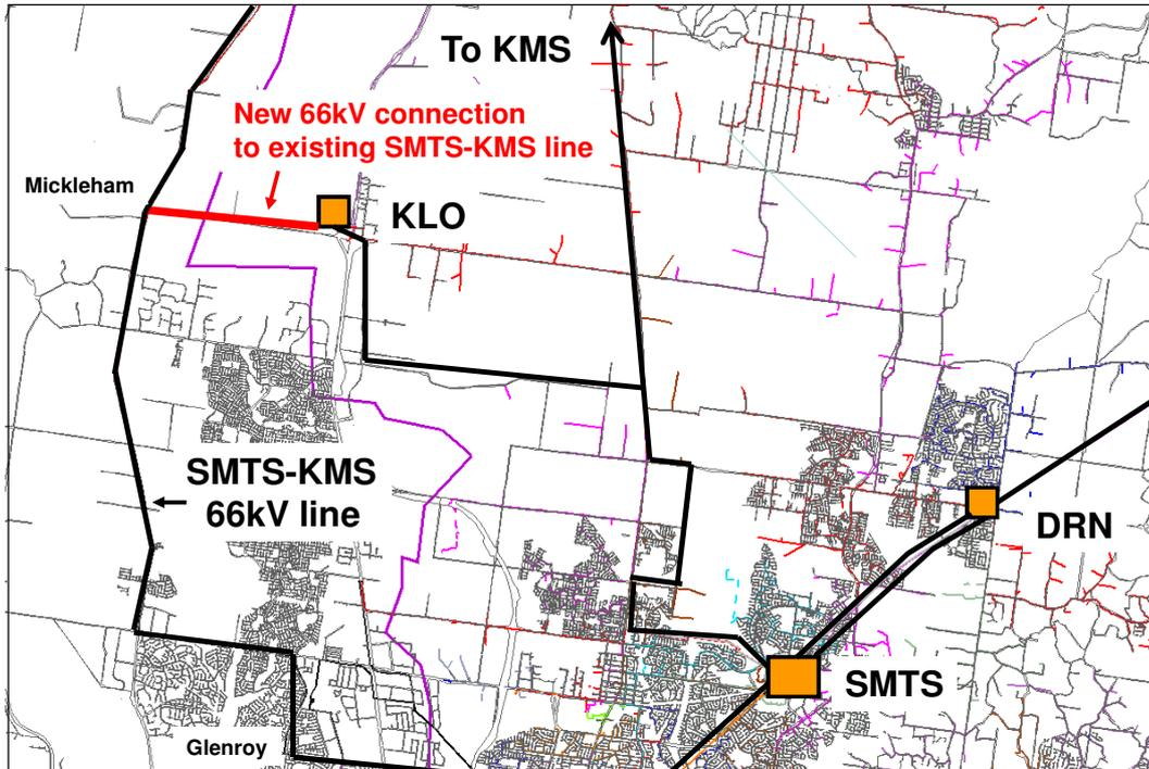
Figure 3 – Connect into existing SMTS-KMS 66kV line to secure second 66kV supply to KLO.
