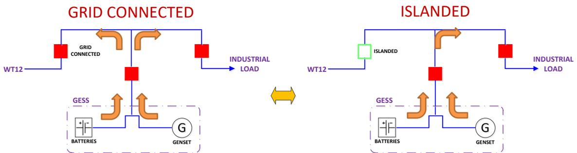
Fig 5: GESS network support modes for grid connected and islanded operation
